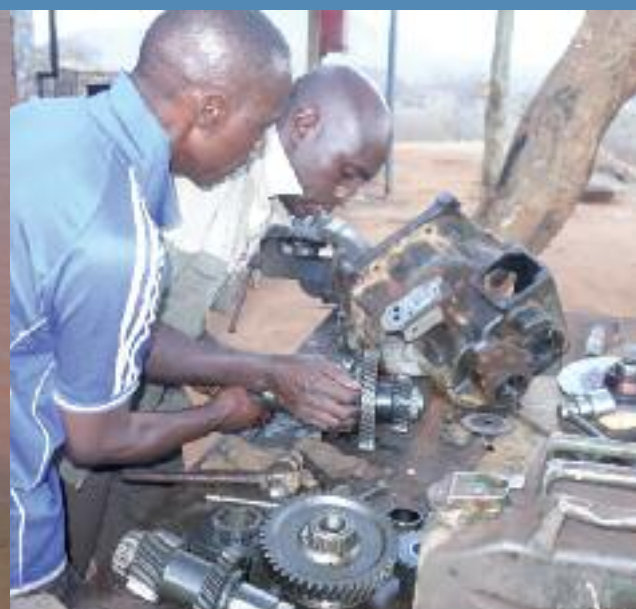
Israel Pallangyo and Fred Ayo make sense out of a JCB gear box
